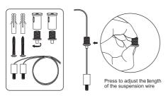
1. Fix hanging rope onto the ceiling.
