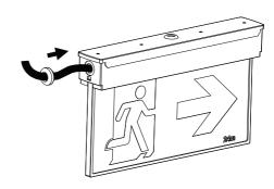
3. Fix the exit sign onto the side mount bracket.
