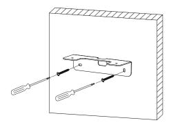
Use a philips screwdriver to fix the back mount bracket onto the mounting surface.
